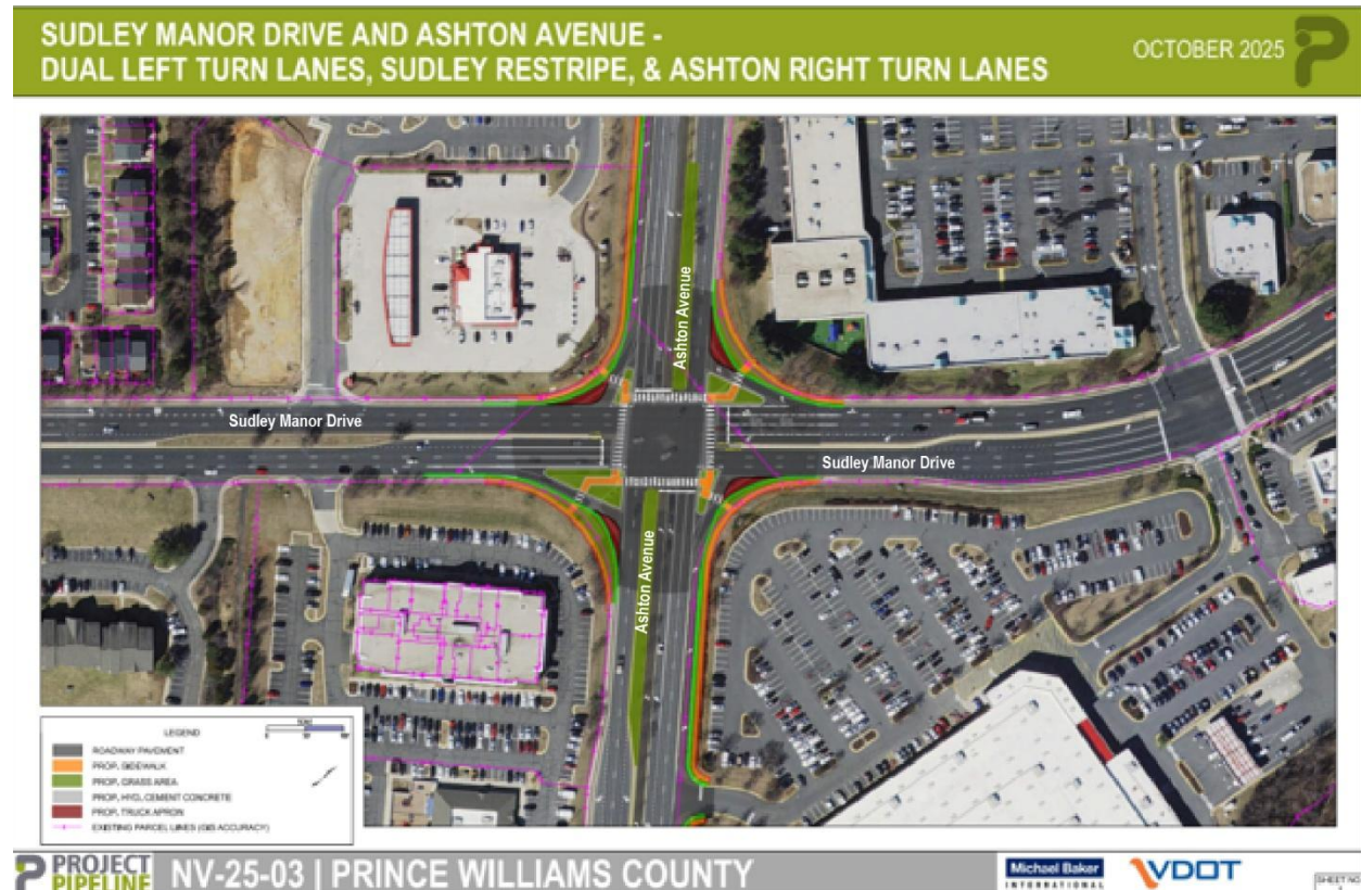
Figure 24: Dual Left-turn Lanes, Sudley Manor Restripe, & Ashton Avenue Right-turn Lanes
