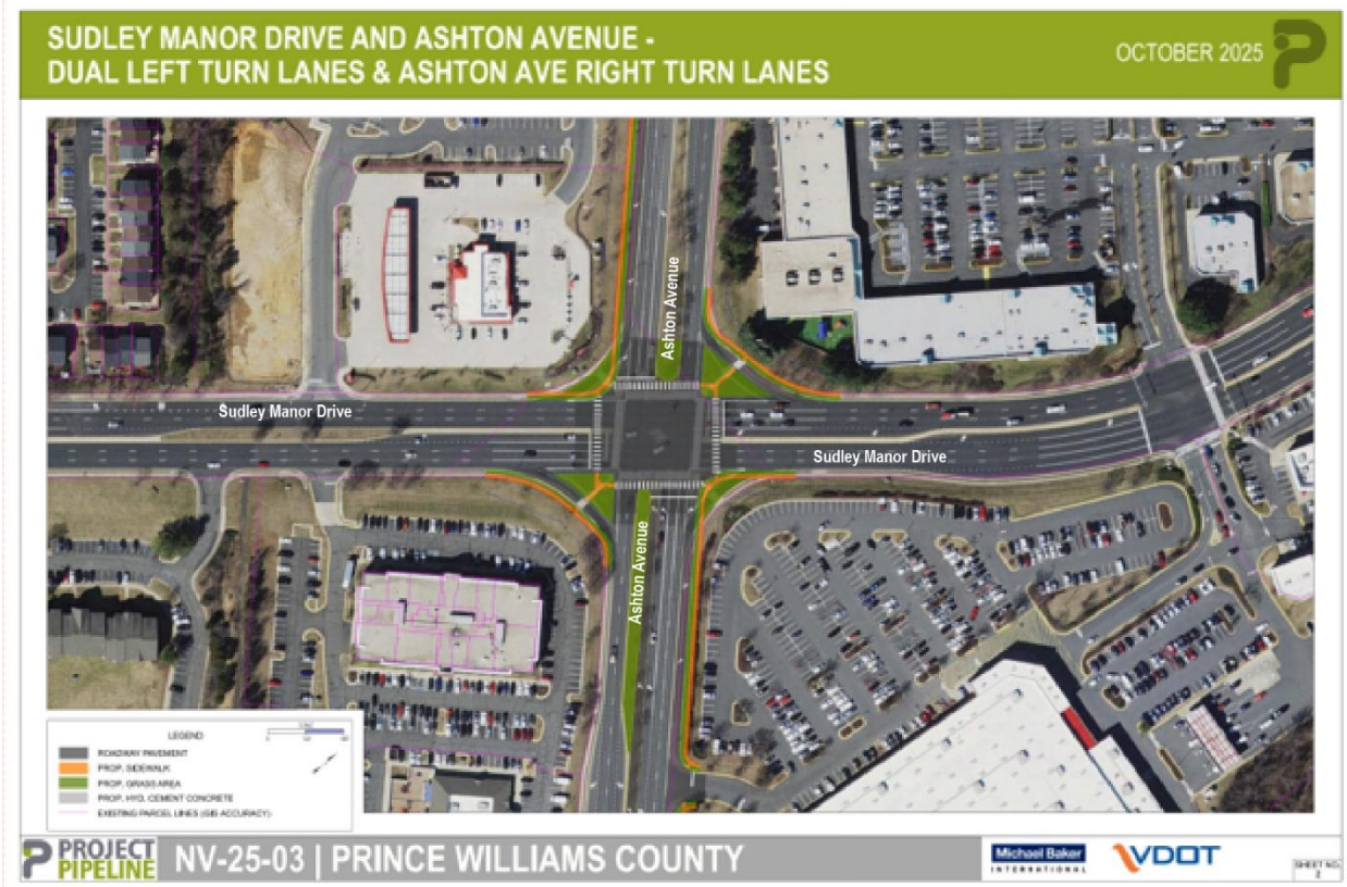
Figure 22: Dual Left-turn Lanes & Ashton Avenue Right-turn Lanes
