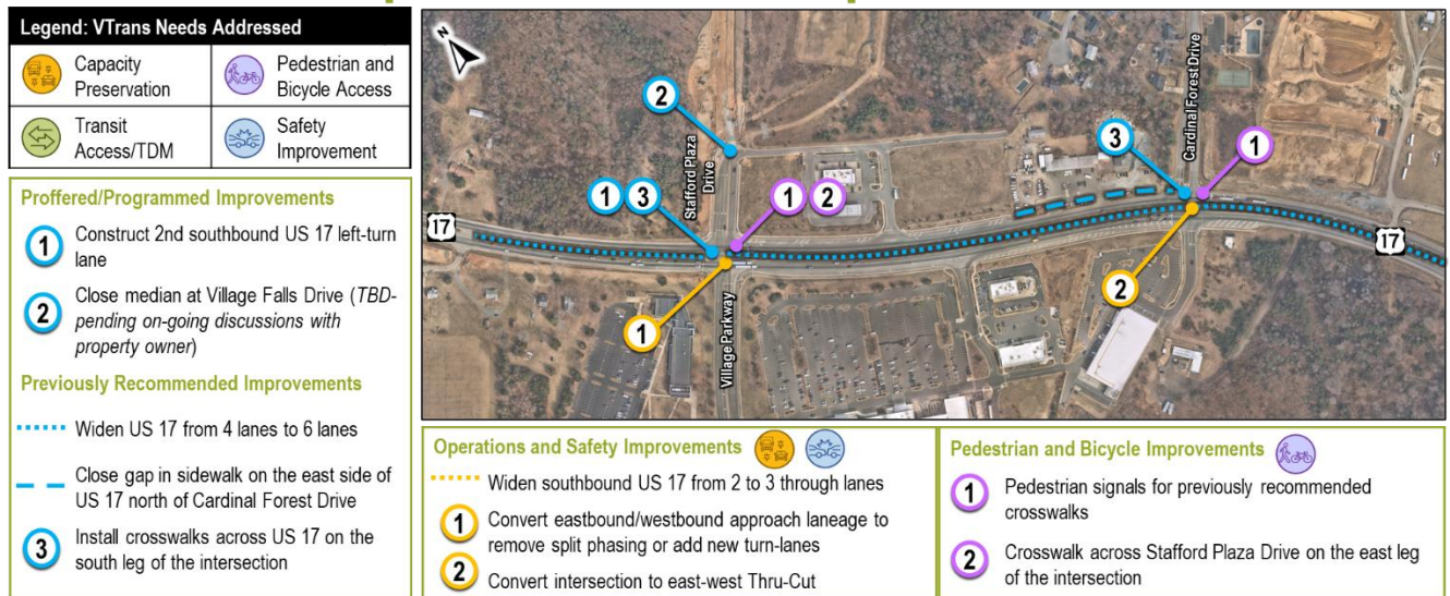
Figure 18: Phase 1 Scoping Level Improvement Alternatives for US 17
