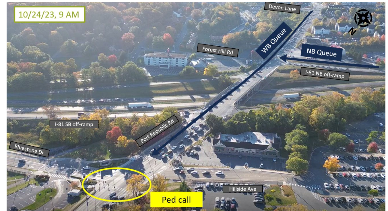
Figure 16. Aerial Image showing areas of significant queuing in the AM Peak Hour
