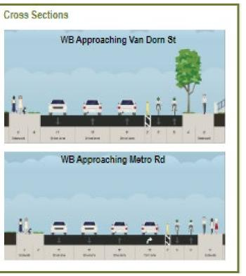
Figure 40: Preferred Alternative Cross-Section
