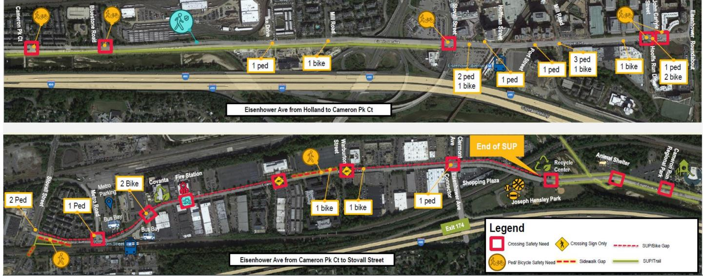
Figure 24. Bicycle and Pedestrian Safety and Accessibility Needs
