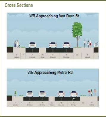
Figure 42: Share-Use Path Alternative Cross-Section
