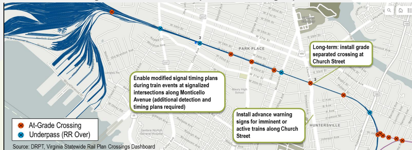
Figure 36: Phase 1 Concept – Rail Crossing Improvements
