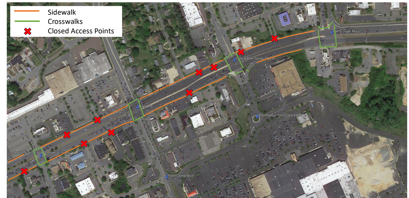
Figure 32: Proposed Pedestrian, Bicycle, & Access Management Corridor Improvements
