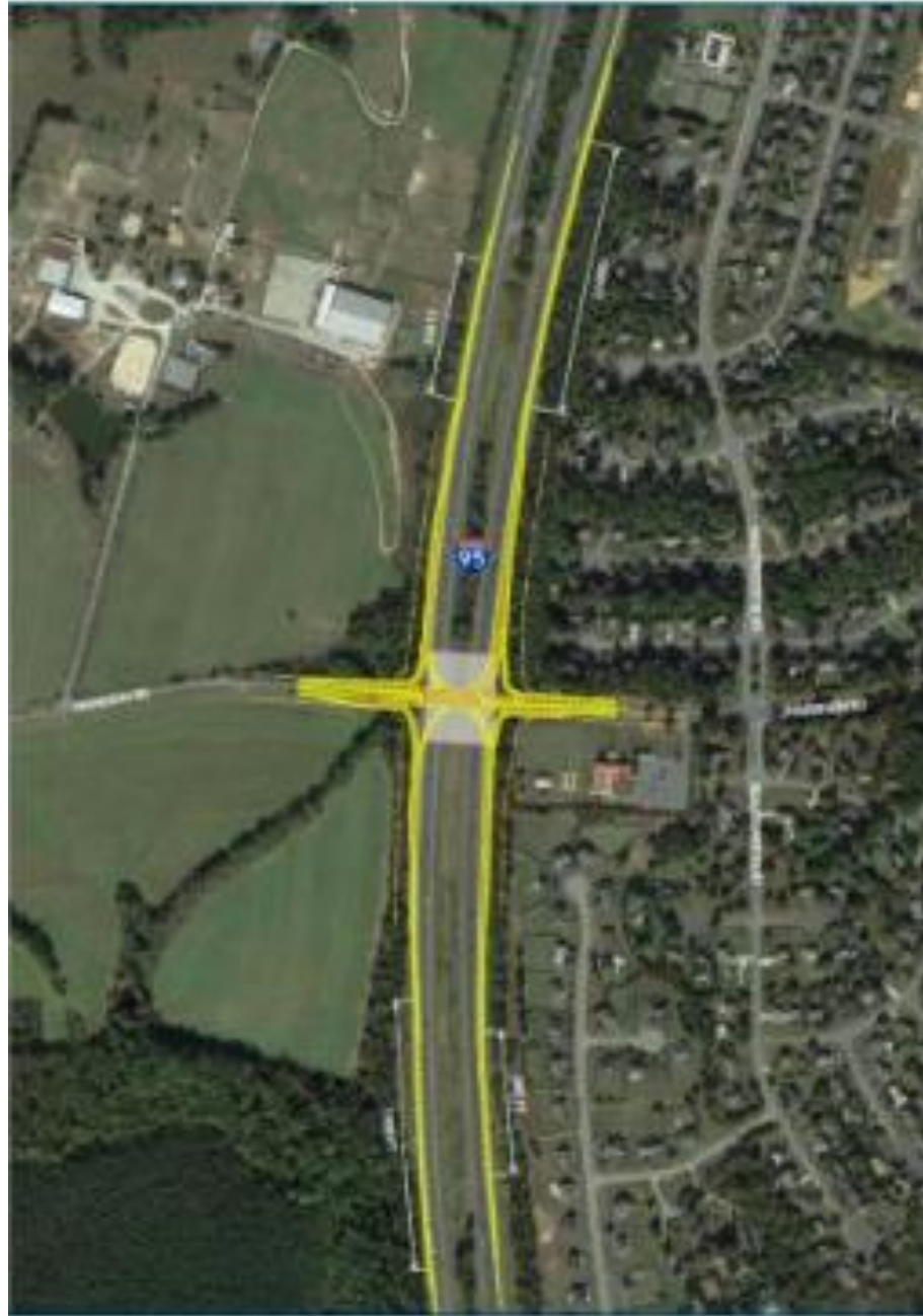
Figure 11: FAMPO Secondary Recommendation - Harrison Road Interchange Concept (Source: FAMPO I-95 Phase 2 Corridor Study Final Report 12/06/18)
