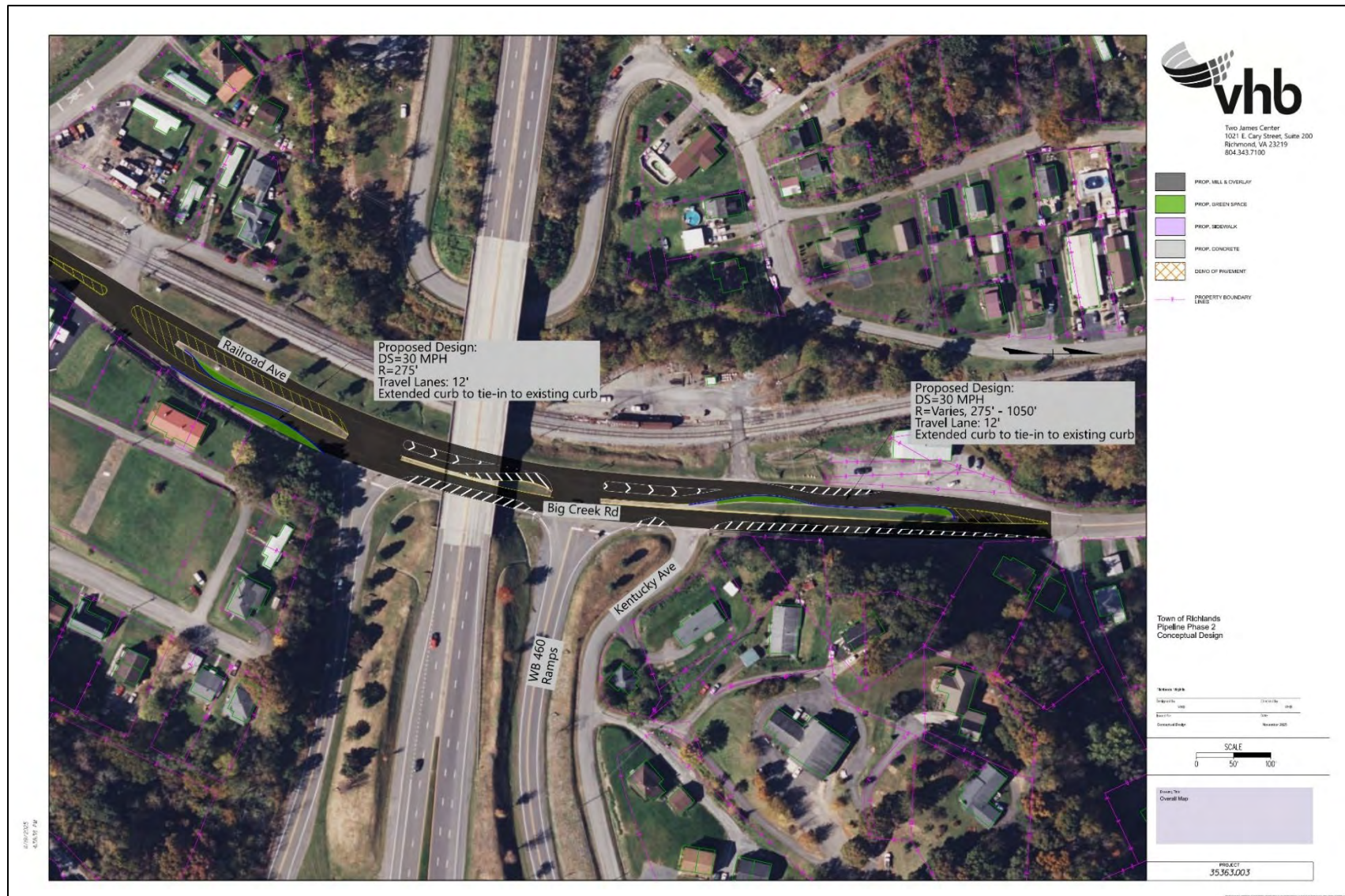
Figure 44: Phase 2 Alternative—US 460 Interchange Chicane
