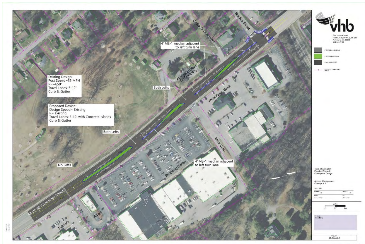
Figure 37: Phase 2 Alternative—Northern Access Management Concept #1
