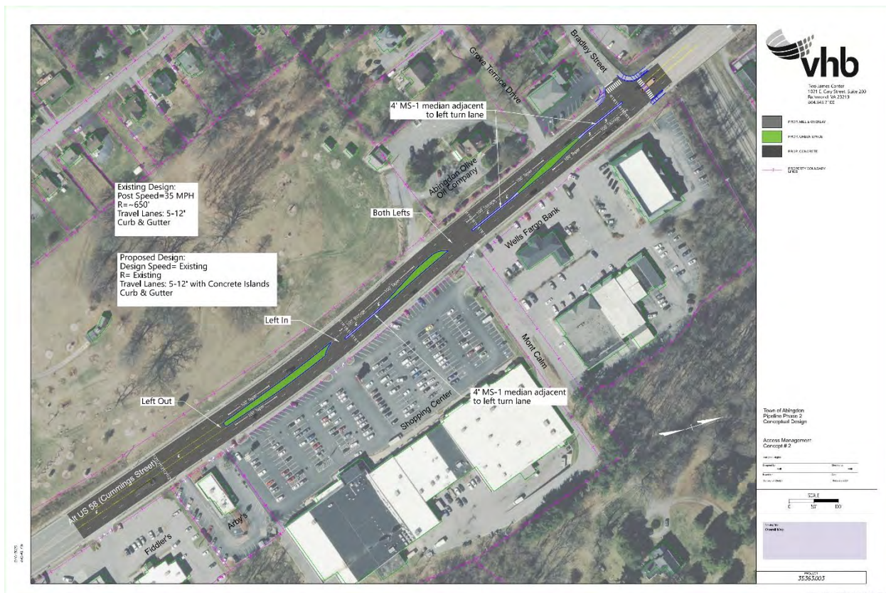
Figure 38: Phase 2 Alternative— Northern Access Management Concept #2
